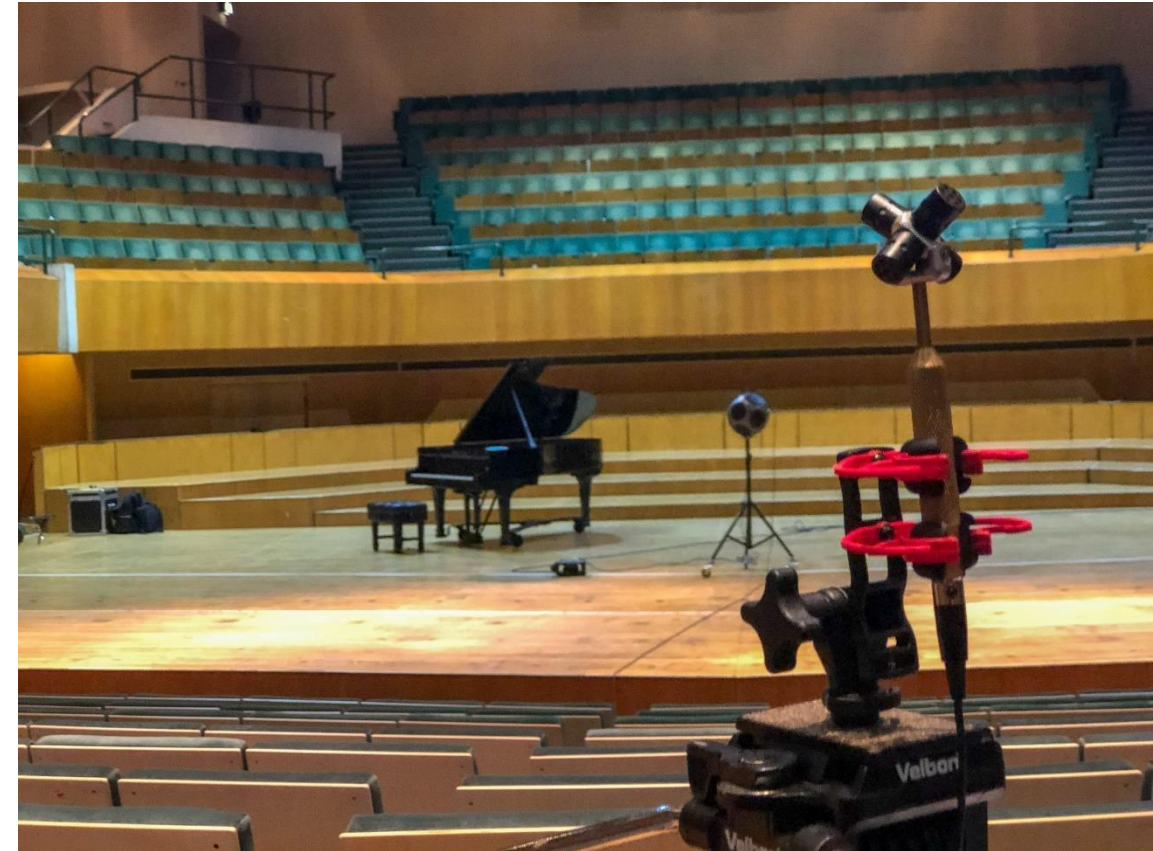
Figure 2 View of IRIS measurement microphone with an omni-directional loudspeaker on stage
